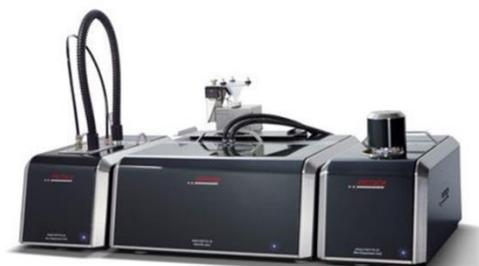
**Fig. 2:** The ANALYSETTE 22 NanoTec was used to measure CBD isolate before & after homogenization. Starting CBD sample (orange) contained a mixture of loose granules with a wide particle size distribution. Material homogenized using the PULVERISETTE 14 classic line variable speed rotor mill (purple) resulted in a particle size consistency similar to talcum powder.
