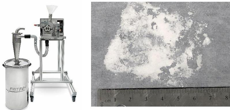
**Fig. 2:** Left - PULVERISETTE 19 cutting mill system, shown with high performance Cyclone collector mounted to 60 L collection tank. Right – CBD isolate homogenized into the low-mid micron range using the P19 system.
